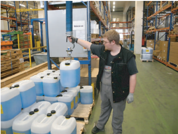
▲ Handling of canisters with mechanical gripper
